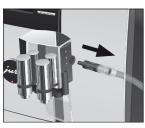
The dual spout must be dismantled and rinsed **daily** if milk has been prepared to make sure it functions perfectly and also in the interests of hygiene.
