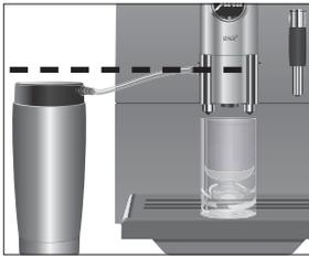
**i** Ensure that the filling height of the milk is **no higher** than the milk pipe connection on the dual spout.
