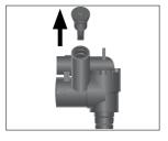
► Remove the air intake pipe.
