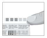
► You will then be able to read the degree of water hardness from the discoloration of the Aquadur® test strip and the description on the packaging.
